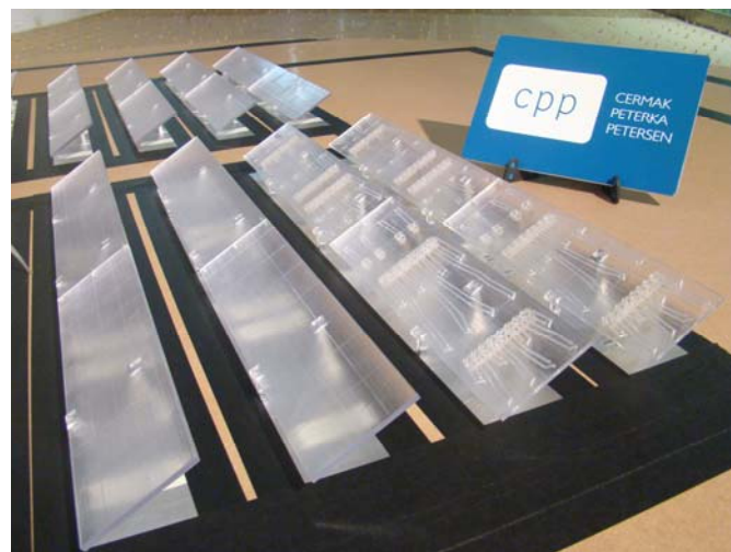
Figure 3: Scale model of PV system on turntable in wind tunnel, showing pressure taps
